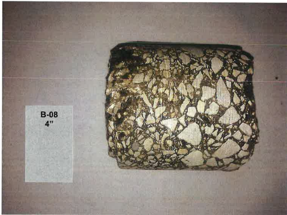
PHOTOGRAPH 22: Pavement core from B-08.
